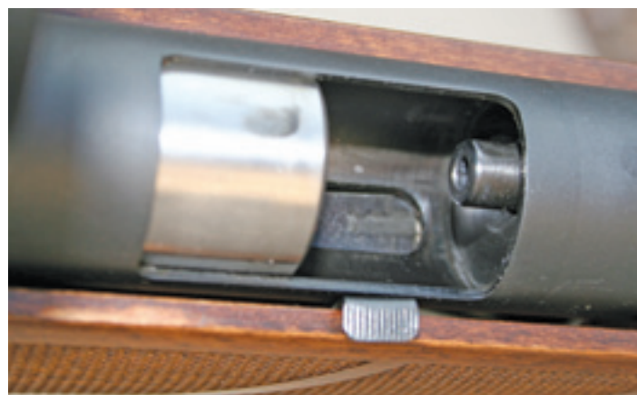
Loading port showing the barrel's breech and, to the right, the release catch that needs to be depressed before the action can be closed
