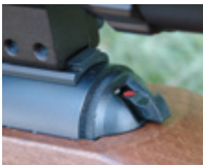
The push/tab safety sits to the rear, but could be broader and less sharp edged for comfort
