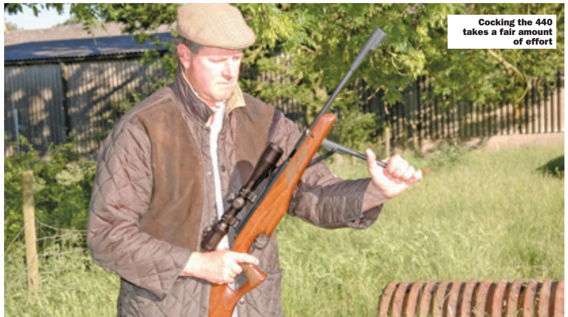
The sliding breech design offers easy hand loading and if you drop the pellet it falls through too
