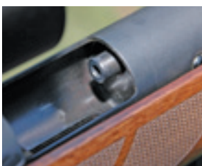
The sliding breech design offers easy hand loading and if you drop the pellet it falls through too
