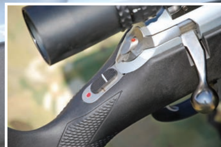
Detail of the practical, tang-mounted safety and the cocked action indicator
