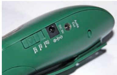
Detail of selector switch that allows both remote and hand operation, note the speaker-out and power-in jacks
